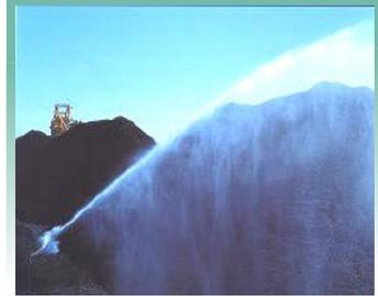
A high frequency drive mechanism provides a fine water curtain and gives excellent water distribution with minimum maintenance. Units can be self adjusting and range from 12 to 150 m<sup>3</sup>/hr with spray trajectories up to 120 metres.
