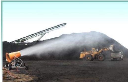
These huge mobile and expensive units can utilise up to 60 hydraulic spray nozzles mounted circumferentially around the outlet head of a large fan assisted barrel. The concentration of nozzle spray together with the high flow of air from the fan, throws the droplets many metres towards the source of the dust activity. The droplets scatter in a plume of relatively soft spray and can capture fugitive dust before it becomes airborne and a major problem.
