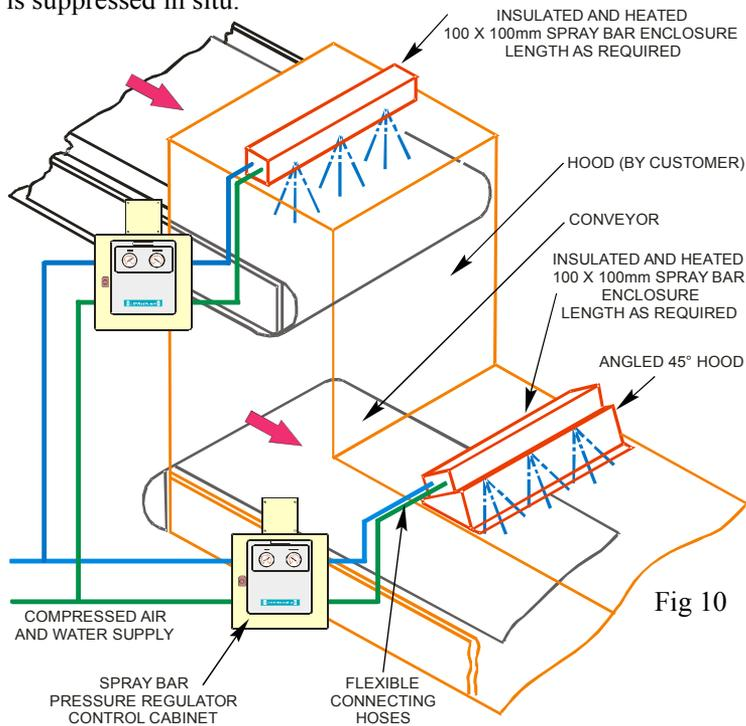
A simple system schematic is shown in Fig 10. In this picture two spray bars are mounted on the covers. They are heat traced and insulated assemblies. The enclosure has a quick release cover, which makes it easy to service the nozzles as required. This picture also shows the regulator control cabinets, which are used to regulate the air and water pressures and would also include solenoid valves linked into the conveyor drives, along with the flex hoses used to connect the two fluids.
